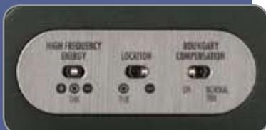
High Frequency Energy, Location and Boundary Compensation switches
